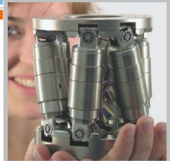
The compact M-810 is smaller in diameter than a CD, but offers long travel ranges in six axes with excellent position resolution
